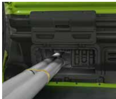
Load through bulkhead flap is magnetised to fix easily and securely in place
