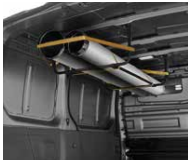
Interior roof rack
